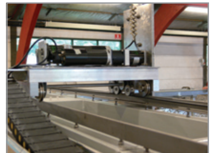
Scanner carriage with motors, brake and gears
